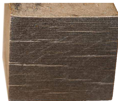
Cut edge of a vulcanised fibre laminate (circa 60 layers / 65mm thick)
