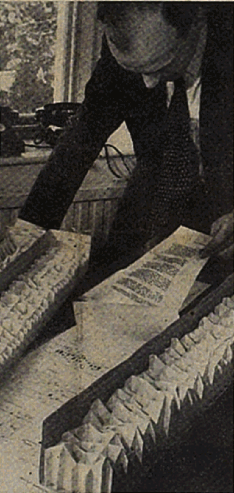
To assist in determining and controlling the product 3-dimensional graphs such as these are constructed to present the relevant statistics obtained from laboratory tests.
